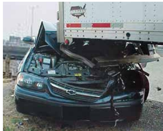
In this 2002 fatal underride crash, a Chevrolet Impala was hit by another vehicle from behind, lost control and struck the back of a tractor-trailer parked on the shoulder.
