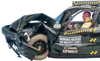
1996 Sonata: Occupant compartment buckled; major intrusion into area around the feet
