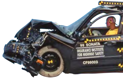
1999 Sonata: Structure improved to marginal; still room for improvement
