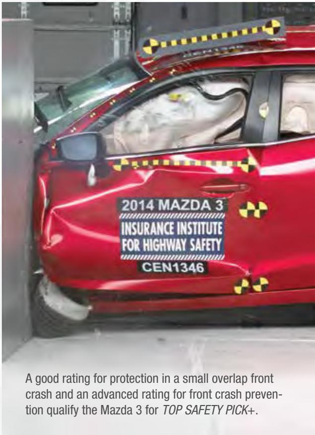
A good rating for protection in a small overlap front crash and an advanced rating for front crash prevention qualify the Mazda 3 for *TOP SAFETY PICK+*.
